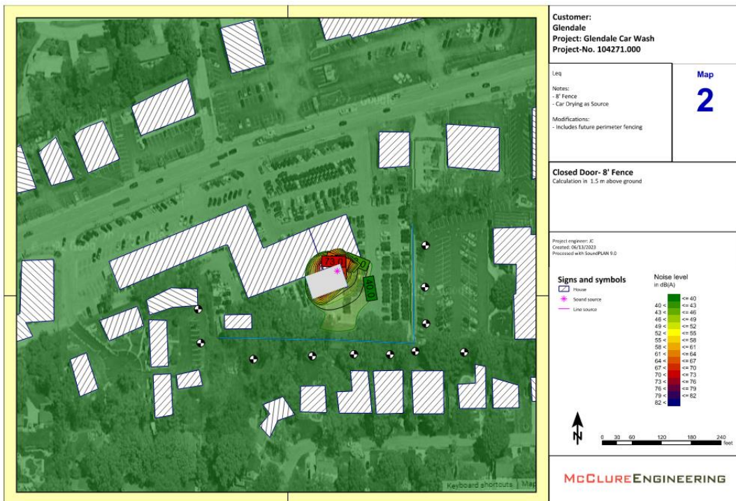
Figure 5 – Sound Map of Carwash Doors Closed (8' fence at PL)– No Background Sound
