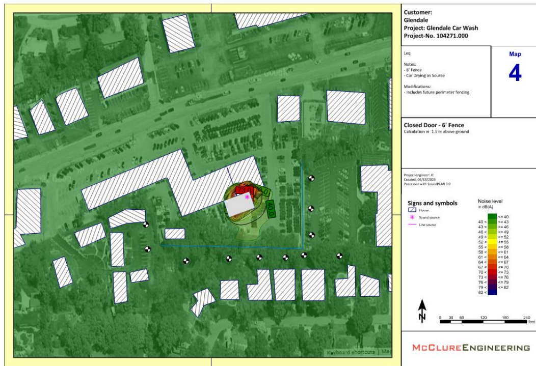
Figure 7 – Sound Map of Carwash Doors Closed (6' fence at PL)– No Background Sound
